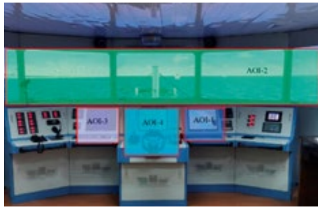
AOIs in the ship pilotage simulations defined by the study authors (Jiang et al., 2021)
